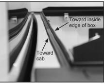
IMPORTANT: Ensure raised portion of seal is against inside edge of box while unraised portion is toward cab.
