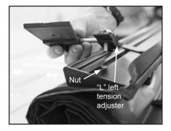
B. Turn 1-1/4" bolt with flat washer onto nut in front bar. Leave loose for now. Repeat for tension adjuster (marked "R") on passenger side of cover and leave bolt loose as well.
