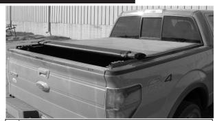
Caution, never drive vehicle with cover unlatched at the rear or partially rolled to the front.
