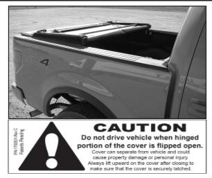
To prevent accidental release of tailgate header, ensure rear header is securely latched to the side rails before driving vehicle.
