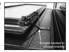
F. Release final latch and carefully tilt cover into storage bracket grooves for vertical position, then secure safety straps to side rails.
