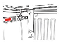
Move the slide block forward to the front bow of the cover.
