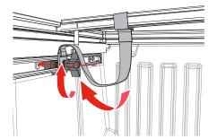
Thread the tether knob through the lock washer, through the tether bracket and into the slide block.
