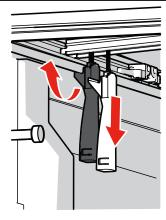
Pull the clamps straight down and release them to hook under the bottom of the metal truck bed rail flange. Always latch the clamps on both sides of the bed.
