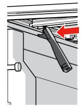
The clamps should be slid, at a slight angle, as far over to the rail as possible.
