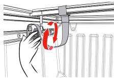
Tighten the knob. Do these steps for both the driver and passenger sides.
