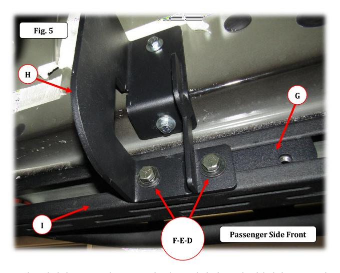
**Step-6** Tighten the bolts securing the mounting brackets to the body panel and the bolts securing the Dominator D6 side step to the mounting brackets.
