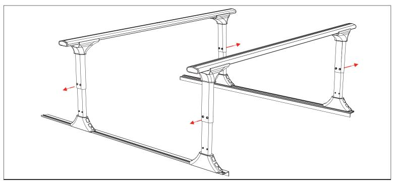
2. Install the Side Bars (#1) to the uprights from the back using 8 Cap Screws (#4), 16 Washers (#6) and 8 Lock Nuts (#5) supplied to accommodate the Side Bars (#1).
