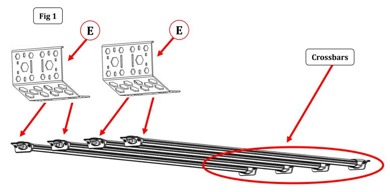
**Step-2** Install and position (3) ¼" x ¾" hex bolts in the center channel of each SRM Rack crossbar or Overland Rack crossbar that will be used for attachment of an Overland Awning Bracket. (Fig 2).
