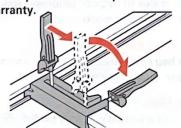
Fold the tonneau forward and fasten the straps in the middle section to the front rail. Check that the straps are tight.
